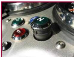
Push the indicator bulb holder up from under the Console and remove lens cap from holder: see the photo, right. Pull the bulb holder down and out from the console. Be careful not to stress the cables.
