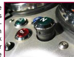
ing. Gently push down on the cap while pulling the bulb holder body from below, until the lens cap sits flush with the Console. A smear of petroleum jelly or silicone grease helps fit the rubber holders.
