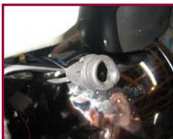
Peel the rubber bulb-holder back over itself to show the bulb seat, as is shown in the photo above. Carefully pull out the old bulb. The bulb can be tight and difficult to remove, in which case it can be lifted using a pair of needle-nose pliers to grasp the base of the bulb, below the round light section.
