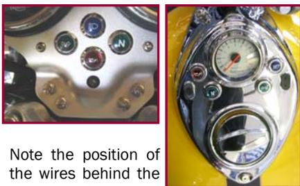
Note the position of the wires behind the speedometer and tachometer. Disconnecting the speedometer drive helps access.
