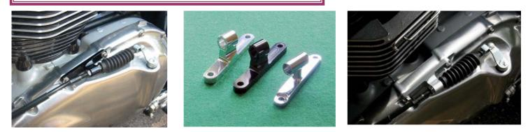
Left:The Black Anodized Aluminum bracket, showing the rubber bellows, supplied.Centre:Close up of the two Aluminum and Chrome BracketsRiahtThe Silver Anodized bracket in place on a Thruxton
